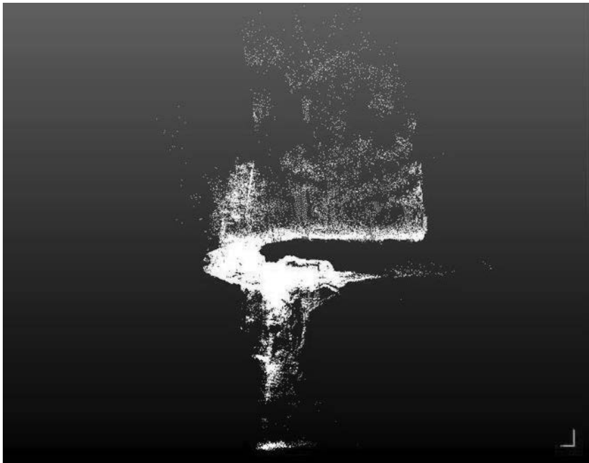
Figure 2: Full extent of the LIDAR data mapping the cave. The data representing the surface above the feature are the points that make up the solid white line with many floating points above it. Points below this line are data representing the caves feature.
