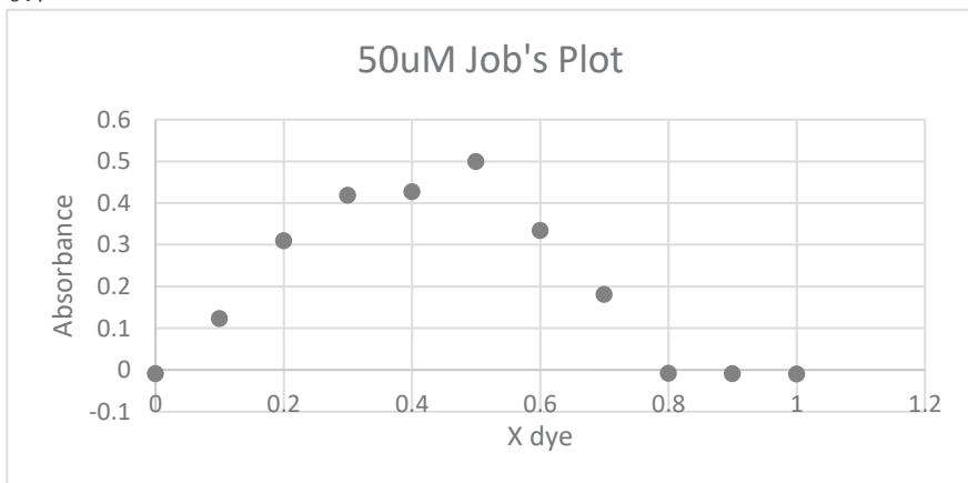
Figure 3. Job's plot for metal-ligand complex between dye 1 and Cr 3+ . Absorbance was measured at 500 nm.
