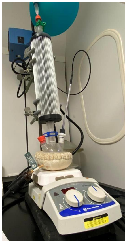
Figure 2. Set-up diagram for the refluxing apparatus.
