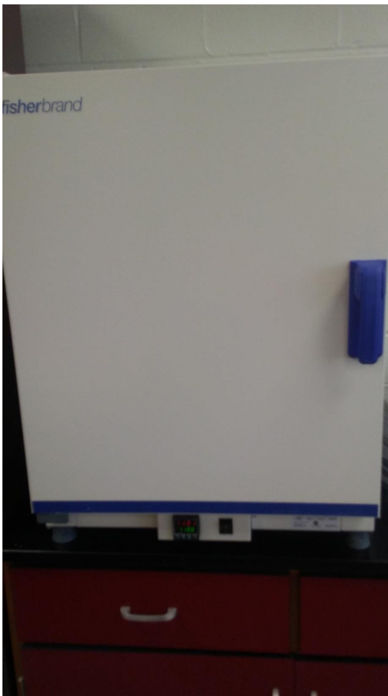
Figure 5: A Fisher Brand oven set to 110 degrees Celsius was used to dry all the glassware and samples after filtration.
