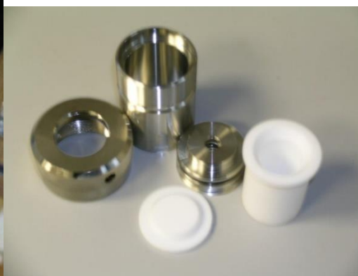
Figure 6: A 1200°C Hybrid Furnace - Tube/Muffle 3-In-1 was used in the hydro/solvothermal synthesis of the coordination polymers in polytetrafluoroethylene-lined Parr 4749 autoclaves with a 23mL internal volume.
