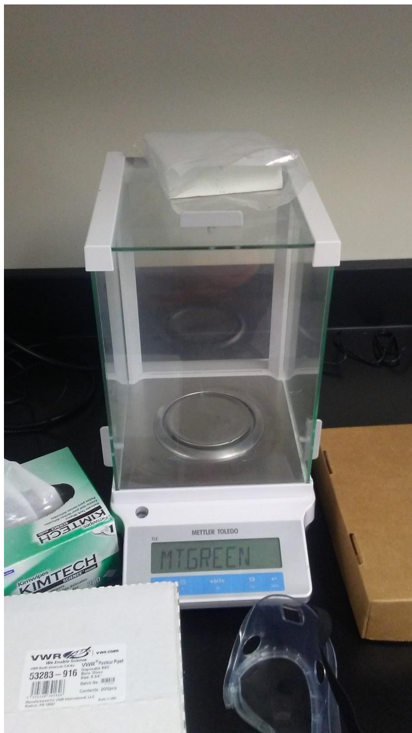
Figure 4: A Mettler Toledo balance with four decimal places was used to mass all the reactants.
